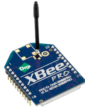
Module ZigBee (ici en OEM : original equipment manufacturer)
